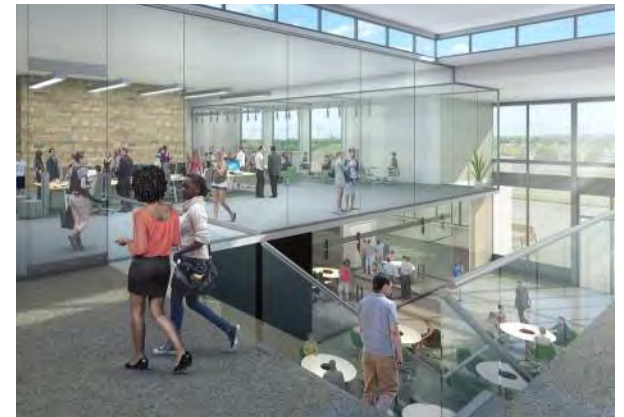
FIGURE 6.35 The Industrial Distribution Building utilizes exterior glazing and clerestory windows to pull natural light deep into the building's interior spaces.
