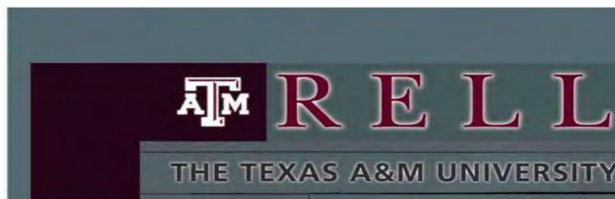
FIGURE 7.13 Primary logo and sub-text cut out of field with halo illumination. Secondary branding element pushed through sign cabinet and internally illuminated.
