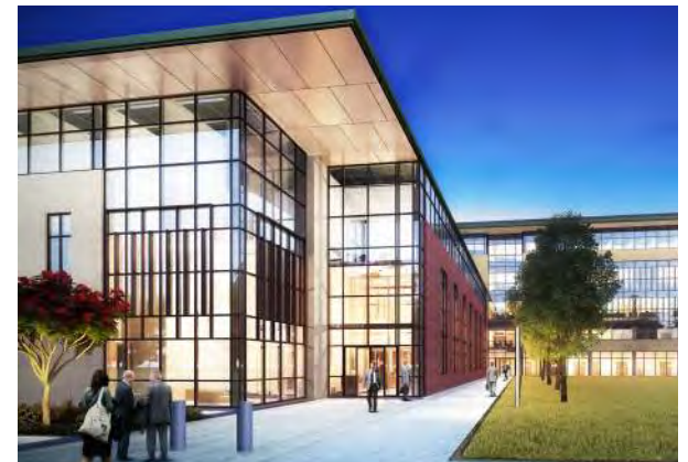
FIGURE 6.39 A deep overhang at the lobby of the TTI Headquarters partially shields glazing from direct sun exposure and keeps water away from the building entrance.
