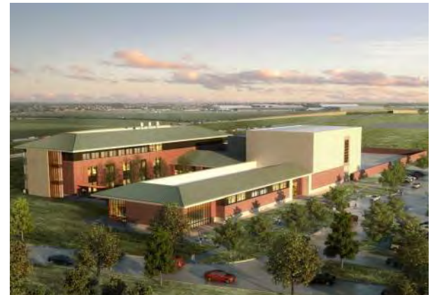
FIGURE 6.43 Mechanical components on the roof of the CIR will be shielded from view at the ground level by partial-height pitched roofs to fit with the campus aesthetic. The loading dock and service yard (at rear) are integrated into the building form and screened by a perimeter wall with the consistent campus brick.
