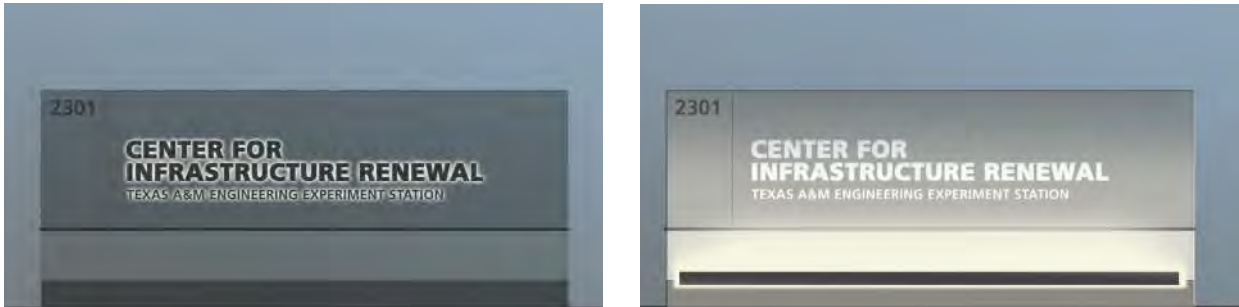
FIGURE 7.54 example of partner monument signage lighting options. internally illuminated, halo lit letters on left; external up-lighting on right.
