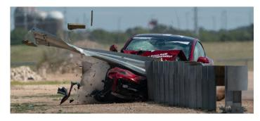
On June 18 TTI and industry leaders convened for a first-of-its-kind crash test in Texas at the Texas A&M – RELLIS Campus. This test subjected a Tesla Model 3 to a 62-mph impact with a thrie beam guardrail system, conditions matching those used in the Manual for Assessing Safety Hardware crash testing. The impact of the crash ruptured the thrie beam rail, allowing the vehicle to penetrate through the barrier. TTI's crash test underscores the importance of ongoing innovation in roadway safety.
