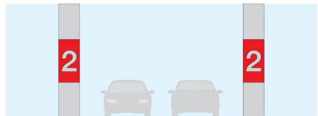
Column Mounted Level Identification
