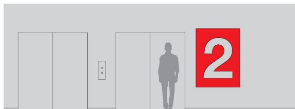
Elevator Lobby Level Identification
